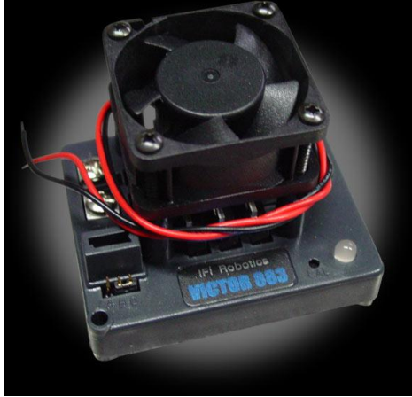
IFI Victor 883- 6-30v, 60a CC, single channel, REV, BRAKE $139.00 ( http://www.robotmarketplace.com/products/IFI-V883.html )
